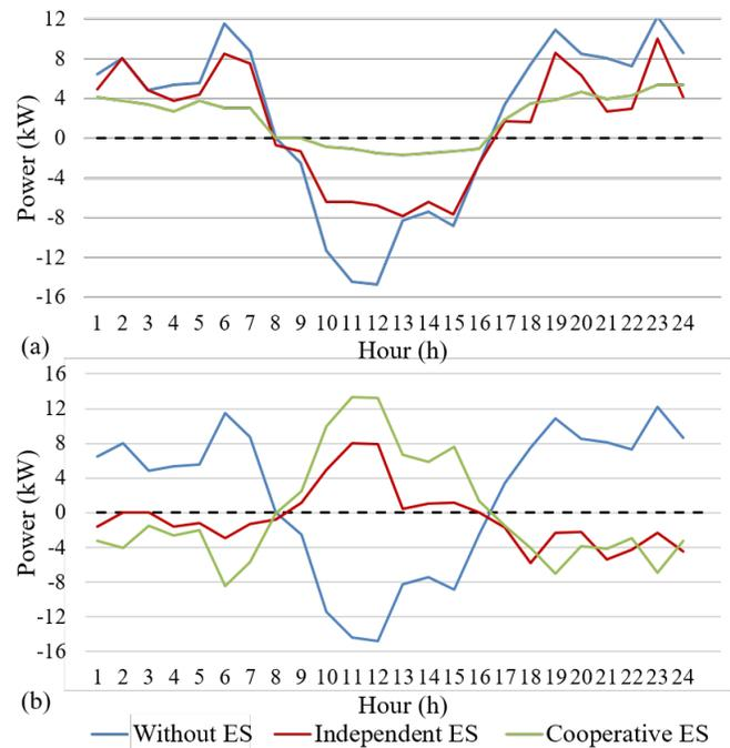
Fig. 4. (a) Net load and generation of the 16-prosumer coalition without ES, with independent ES operation, and with cooperative ES operation; (b) Aggregate ES charging and discharging scheduling with independent and collaborative ES operations.
